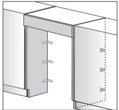
screw the unit to the wall behind using a number of suitable angled fixing brackets. Use suitable wall plugs/fixing screws for the type and material of the wall.
